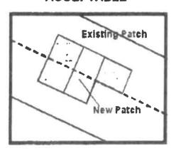
3. Asphalt and concrete pavements should be removed by saw cutting or grinding. Avoid breaking away the edges of the existing pavement or damaging the remaining pavement with heavy construction equipment.
