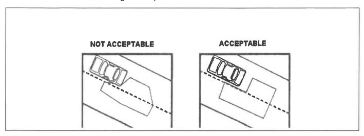
2. Avoid patches within existing patches. If this cannot be avoided, make the boundaries of the patches coincide.
