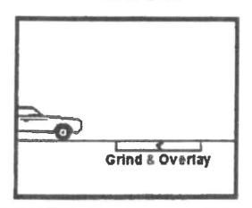
iii. Surface tolerances for street repairs should meet the standard for new construction. That is, the finished surface of the street repair, when tested with a ten (10) foot straightedge parallel to the centerline or perpendicular across joints, will show variations measured from the testing face of the straightedge to the surface of the street repair which do not exceed one-quarter (1/4) inch.
