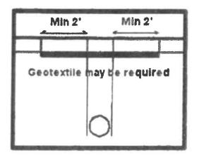
2. For patches in asphalt, a tack coat shall be applied to all edges of the existing asphalt before placing the new pavement. After placing the new asphalt, all seams (joints) between the new and existing pavements shall be sealed with an asphalt tact coat or rubberized crack seal material. (Ord. No. 305, 2008)
